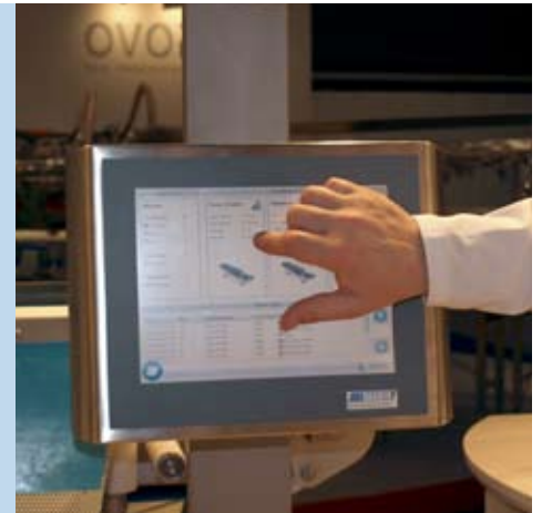
Step 6: Weighing the fillets on LINCO-flex Easy Grader. At the terminal it is possible to manually enter production events such as lack of raw material, lack of operators or machine downtime
