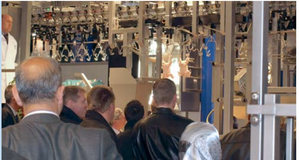
Step 2: The chickens are loaded onto the ProFlex Premium Cut-Up line. At this demo the Vision Quality Classification is mounted on the cut-up frame but in real life it can be placed anywhere after the evisceration.
