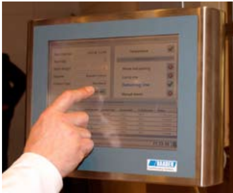
Step 1: The weight of the whole chicken is entered into the system. At the plant the information comes from a weigh transfer or a weighing bridge.
